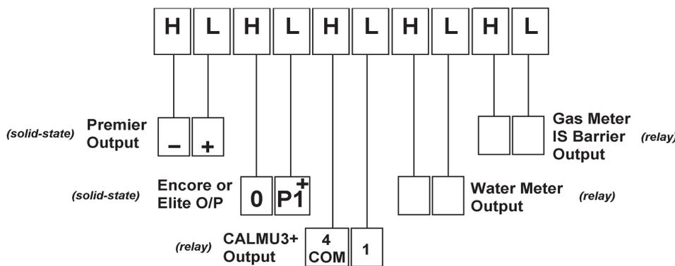
The datalogger input channels are wetted with a dc voltage. Polarity must therefore be observed when connecting to devices with solid-state outputs, such as Sprint, Premier, Encore or Elite meters.
