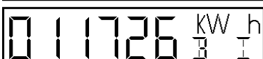
Billing register for kWh import, in this case showing 11726 kWh. The contents of the main energy registers are copied into the billing registers at each billing point. The billing registers remain 'frozen' at the most recently billed value until the next billing point. (Only on model EN305).
