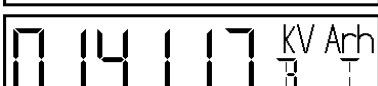
Billing register for import kvarh (lagging for active import energy), in this case showing 14117 kvarh. (Only on model EN305).
