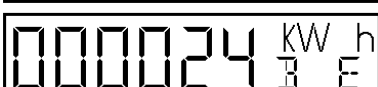
Billing register for kWh export, in this case showing 24 kWh. (Only on model EN305).
